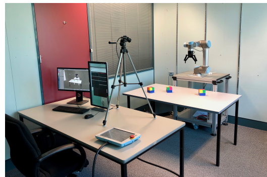
Fig. 5. Lab environmental set-up. The end effector shown is at the default home position. The camera’s optical centre, table surface centre, and UR5 base joint are aligned.
