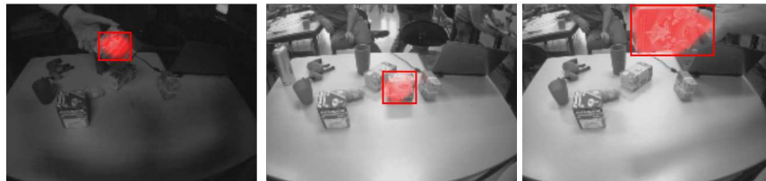
Figure 1-5. Examples of an evolved filter running in real time on the iCub. Considering the limitations of the training set (Figure 1-4), the evolved filters show good ability to generalize to variations in lighting, scale and rotation.
