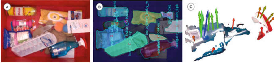
Fig. 6 The perception pipeline, showing (a) RGB image of items in our storage system, (b) output of semantic segmentation, and (c) segmented point cloud for the bottle, with grasp points calculated (higher ranked grasp points shown as longer and green and the best candidate in blue). Even though the semi-transparent bottle results in inaccurate depth information, our system still finds good grasp points on the centre of the bottle, with points on the neck and head being weighted lower
