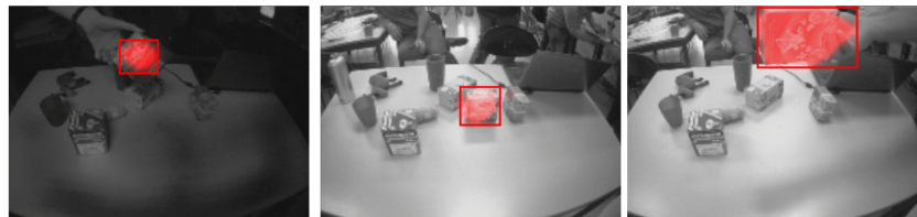
Fig. 2 The detection of a tea box in changing lighting condition performed by a learned filter. The binary output of the filter is used as red overlay.
