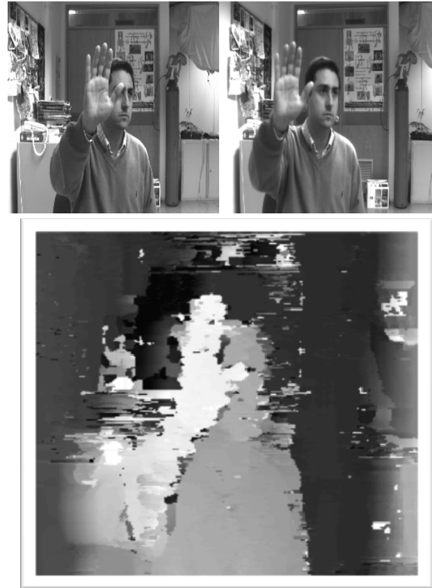
Figure 4: A sample disparity map corresponding to the stereo pair in the top.
