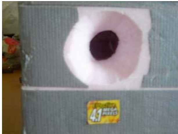
Figure 5: Camera Hole in the REEL insulation
