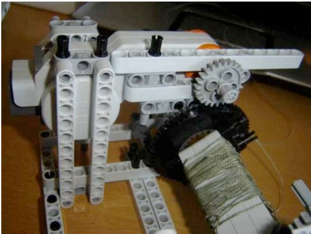
Figure 4: The mounting of the reel with the motors and the supporting structure
