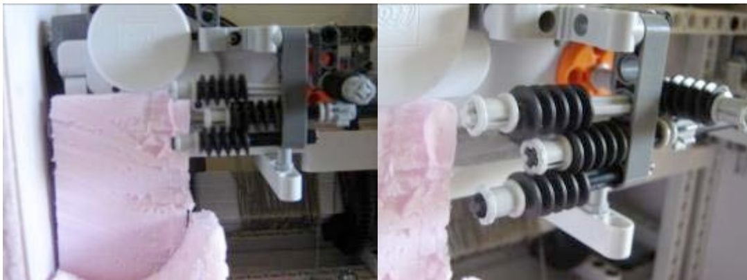
Figure 6: The camera cradle made out of insulation (left) and the shooting mechanism (both) using the locking-system motors
