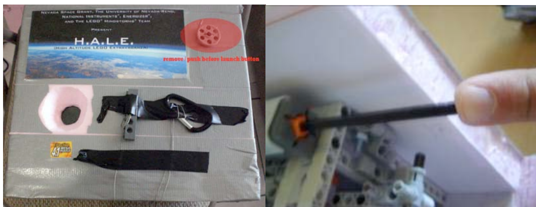
Figure 7: Press-Before-Launch Button (external and internal view)
