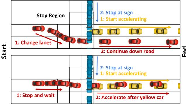
Figure 3: Two different solutions to safely passing through an intersection. The red car is using the proposed algorithm. Top: manual high-level policy changes lanes, bottom: learned high-level policy waits for car in front.
