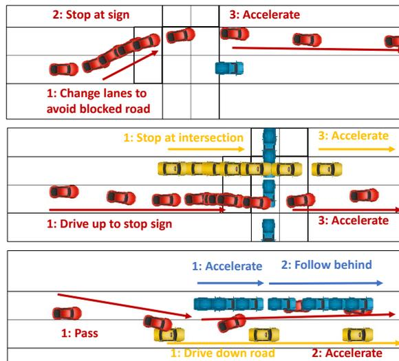
Figure 1: Simulated self driving car problems containing an intersection and multiple vehicles. The car must be able to behave intelligently when confronted with sudden obstacles like stopped or slow moving vehicles, and it must be able to obey the rules of the road.
