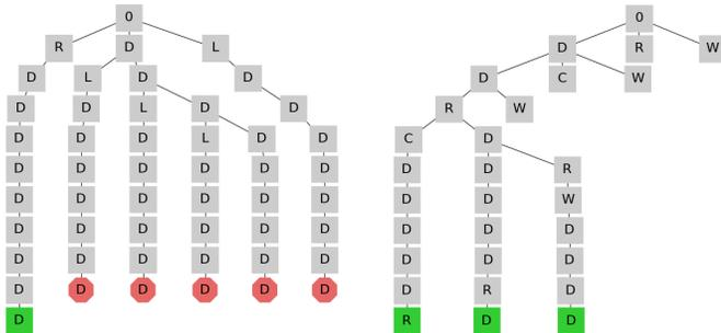
Figure 4: Comparison of MCTS on a test problem with a stopped car. Letters indicate option being executed: 0 = root, D = default “stay in lane” policy, W = wait, C = finish level, R = lane change right. On the left is tree search with a manual prior over options; the right tree uses the learned high-level policy. Green leaves indicate success; red leaves indicate failure.
